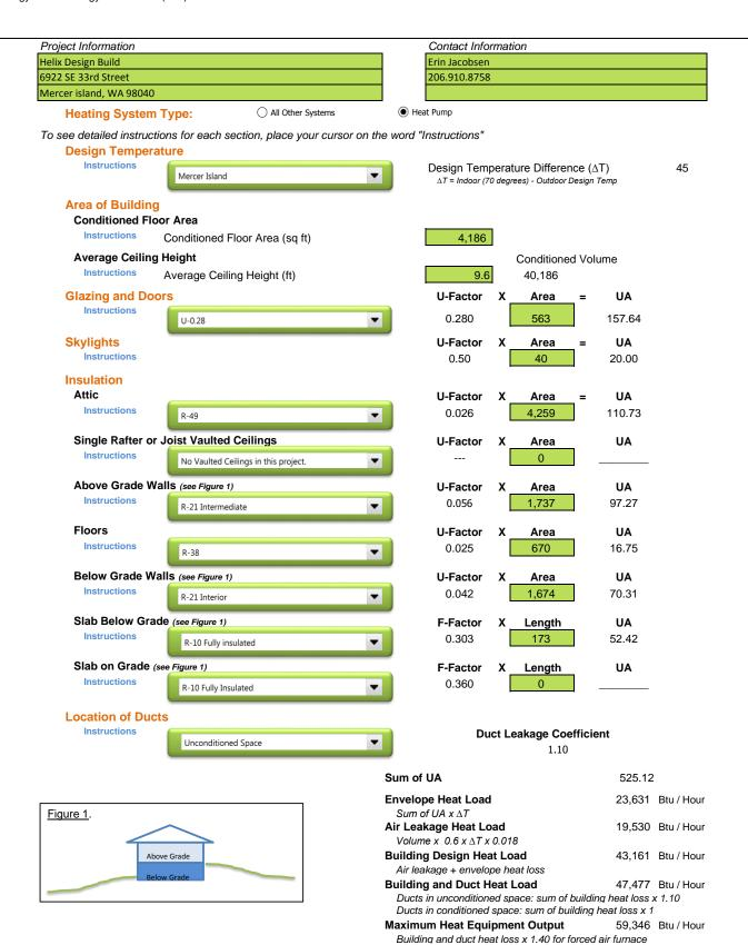
Building and duct heat loss x 1.25 for heat pump
